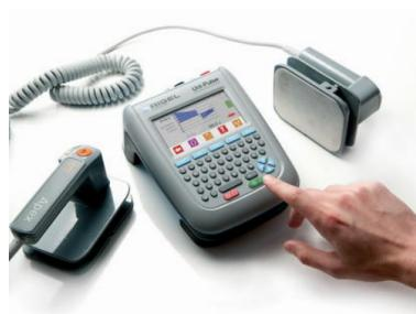
**ANALIZATOR ELEKTROKIRURŠKOG GENERATORA**
