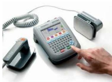
**ANALIZATOR ELEKTROKIRURŠKOG GENERATORA**
